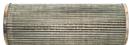
Oil screen: No plugging or debris.
