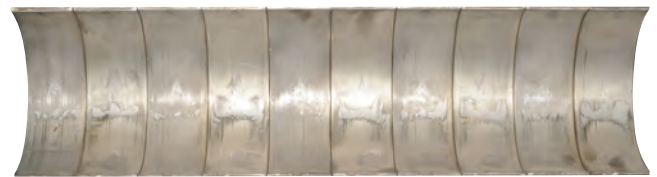
Upper rod bearings: Light to medium scratching with cavitation, except for two that had no cavitation.
