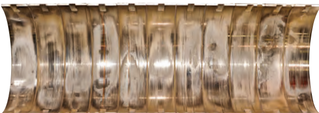
Lower main bearings: Light to medium scratching except in two that had heavy scratching w/ <1% and ≤10% exposed copper.
