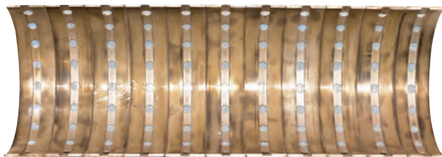
Upper main bearings: Light scratching, 0-20% overlay removed.
