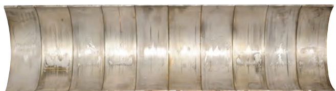
Lower rod bearings: Trace to light scratching.
