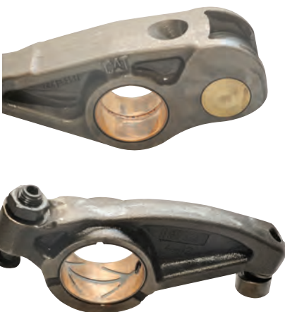
Exhaust/intake rocker bushings: No visible distress noted on any of the rocker arms. Bushing wear as follows: Average overlay removed: injector 20%; intake and exh <5% w/trace to light wear.
