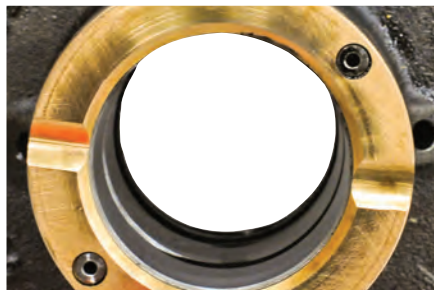
Thrust bushing: Light wear and scratching.
