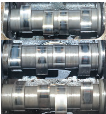
Camshaft lobes: Trace wear, some pitting on several but no worse than trace. No wear step was detectable on any lobe surface.
