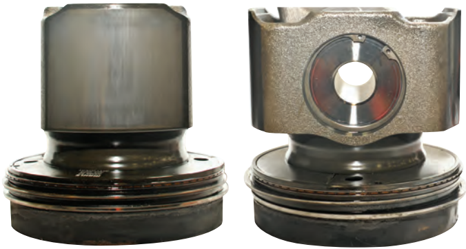
Pistons, rings and liners: Trace scratches on liners with some staining. Minimal bore polish (<5%) on liners. No signs of scoring on thrust or anti-thrust sides.
