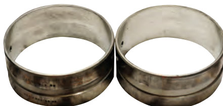
Cam bearings: No signs of distress or wear.
